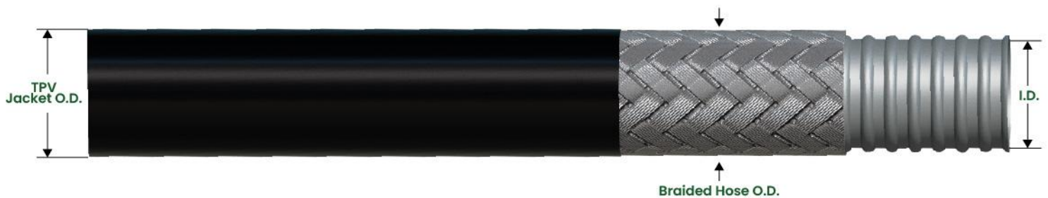
Figure 1 - Extruded Hose Dimensions
